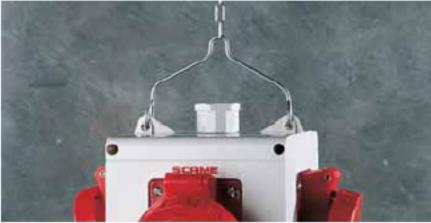
In all installations where the power supply must come from above (for example in the workshops of carpenters or other trade workers), the adaptor can be hung from its handle by a chain or metal cable. In this way mechanical tensile stresses are not passed onto the electrical supply cable.
